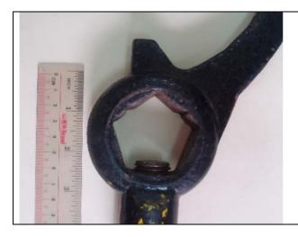
The hydrant key is also used to open the following valves. A pentagon valve up to 1¾ inch and a square nut valve up to 1¼ inch.
