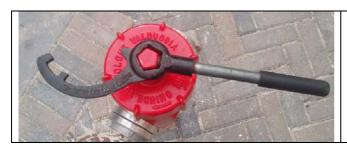
This adjustable hydrant key fits the valve, which is located on top of the hydrant. The hydrant key is used to open and close the water flow. The hydrant key is also used to open the blind Storz covers.
